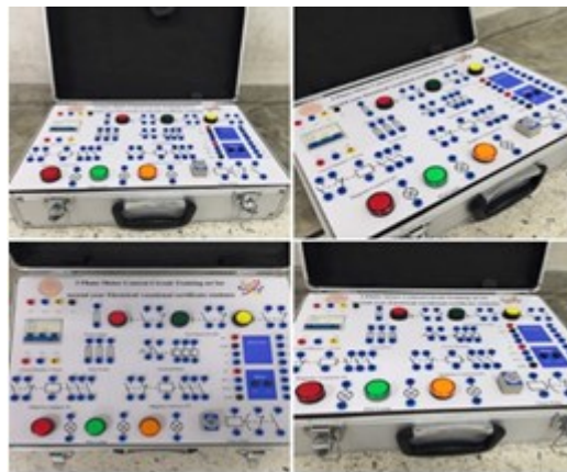
Fig 4. Three-phase motor control circuit operating set
