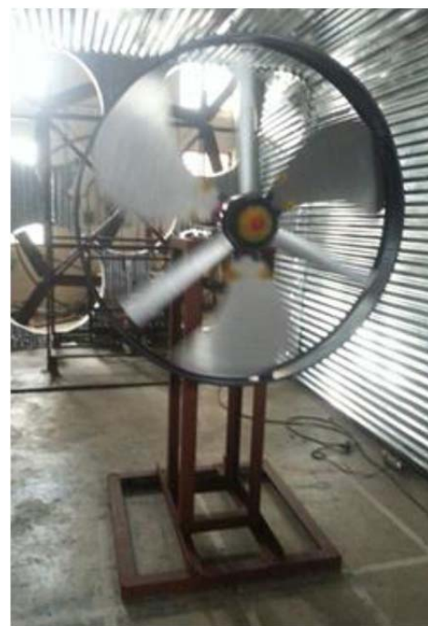
Fig. 4. a) Low-wind-speed wind tunnel and b) The CWTB testing in the wind tunnel
