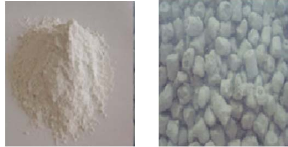
(a) Original mineral talcum (b) Mineral talcum pellet
