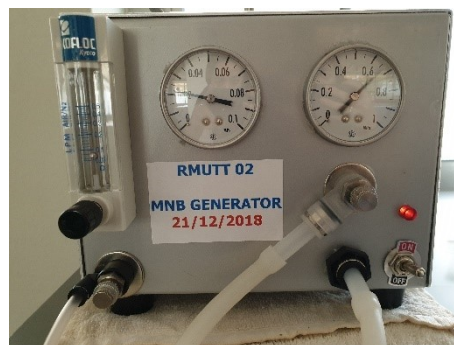
Fig. 1. RMUTT-MNB generator developed for basic research at RMUTT.
