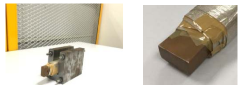
Fig. 18 Model 2: Defect on insulation of endwinding.
