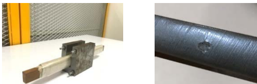
Fig. 20 Air gap on outer layer.
