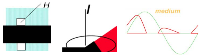
Fig. 9 Surface discharge between bus and air insulation.
