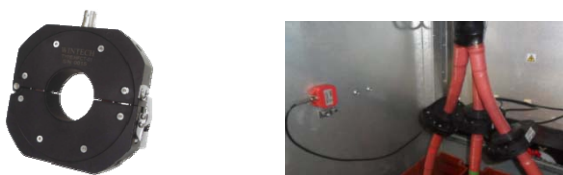
Fig. 14 HFCT Sensors and installation.
