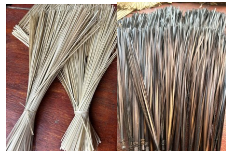
Fig.1 Characteristics of bamboo stripes: (left) not exposed to smoke and (right) that have been smoked.
