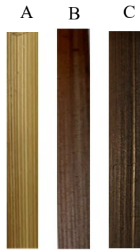
Fig. 6: Color of Bamboo strip: A) Unexposed to smoke; B) Traditional smoke oven smoked; C) Developed smoking kiln smoked.
